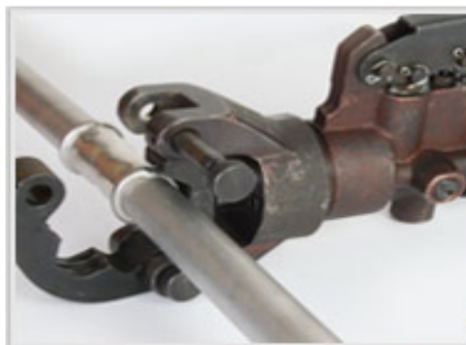
Open the jaws of the pressing tool and insert the assembled tube and fitting to be pressed
