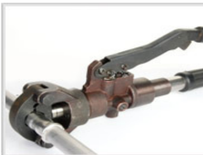
Press the lever and make a joint
